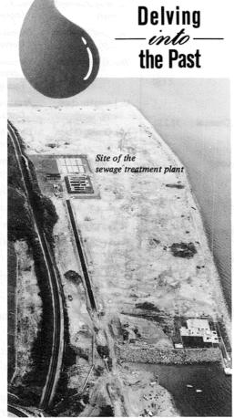
purify the waste water coming mainly from the toilets. Incoming sewage from all over the campus was directed through drains to the new plant. After the various purification processes of grit removal, primary sedimentation, aeration and comminution, the water quality would be of a high enough standard to be discharged, through an underwater pipe, into Tolo Harbour.
